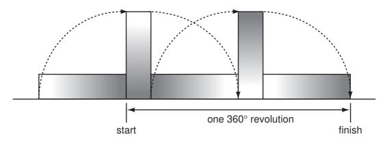
It is quicker to lower a tall stone than to raise it. From experience, a stonemason knows that he can turn a stone through 90° in (b/h) minutes, where *b* is the length of the face that is flat on the ground, and *h* is the vertical height of the stone as he is about to turn it.
